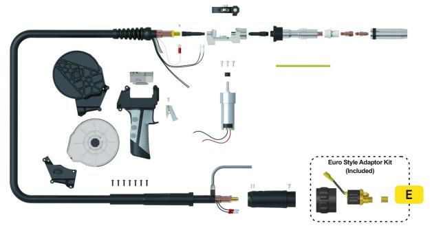
By using one of the following adaptor kits, the termination type of this MIG gun can be changed to another widely used termination types.
